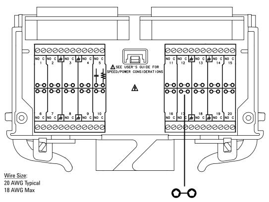
Pads for user-supplied snubber circuity to alleviate reactive transients. The circuits may consist of resistors, capacitors, varistors, or other elements as needed to reduce the switching voltage and current transients inherent in reactive circuits.
